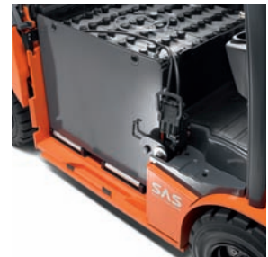
Battery side extraction with roller bed
